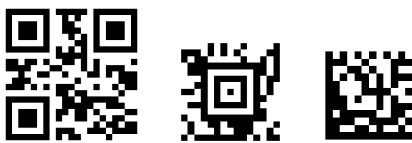
Figure 5. Popular 2D Barcodes with rectangular pixels: Quick Response, Aztec, Data Matrix
